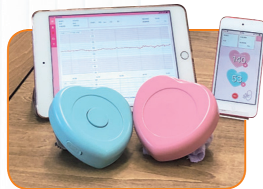
Left: The Petit CTG is simple to use, providing OB/GYN professionals with the fetal heart rate remotely, and almost in real time. Bottom: The heart-shaped Petit CTG comes in blue for the mother's cardiocotography, and pink for the baby's.
