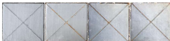
One-component type of zinc paint with 7% HAp
