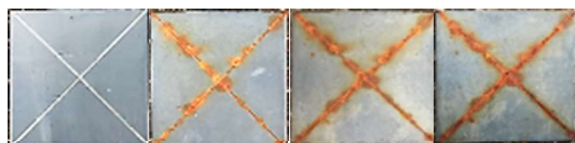
One-component type of zinc paint without HAp
