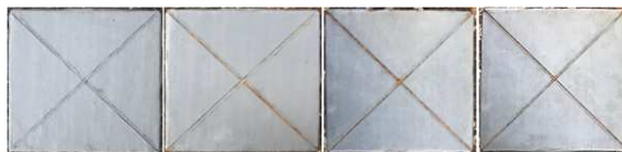
One-component type of zinc paint with 7% HAp
