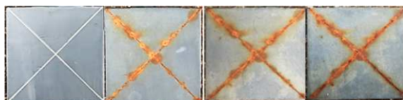
One-component type of zinc paint without HAp
