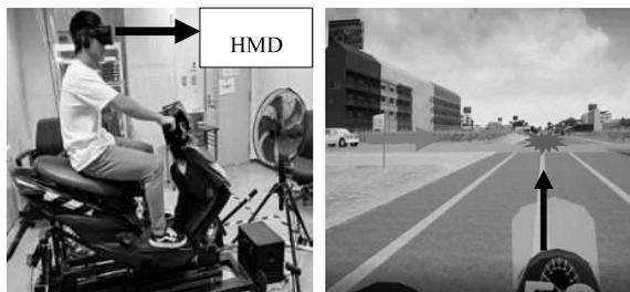
Figure 1: a) Riding simulator b) Experimental scenario
