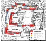
Location of deformed wall and the distribution of the thresholded value of H/H ratio by microtremor
