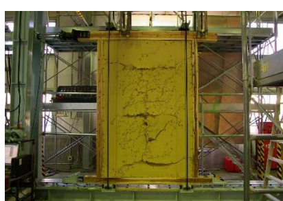
Fig. 5. Static Test for Mud Wall
