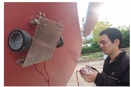
Wall Climbing robot by Magnet Adhesion can move on the vertical wall by adsorbing on the steel wall
