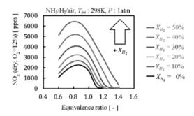
Fig. 2 The effect of X<sub>H₂</sub> and equivalence ratio on NO<sub>x</sub> emission level.
