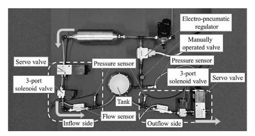
Figure 7. Experimental setup of multi-layered variable volume tank.
