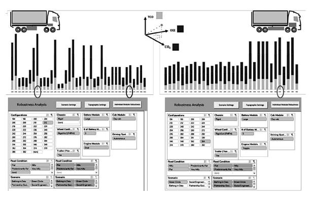
Figure 8 Snapshot of the scenario evaluation model highlighting top performing vehicle configurations across all scenarios(left) versus only one (Green Circle) scenario (right)
