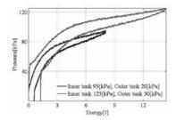
Figure 5. Energy characteristics of multi-layered variable volume tank
