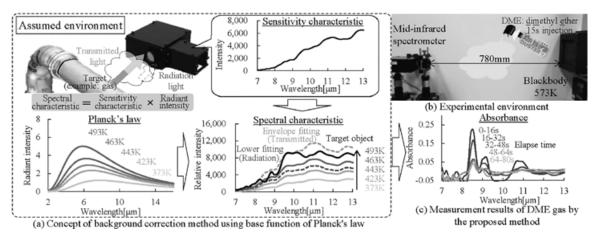
Fig. 1 Planck's law base-function for background correction and measurement results of DME gas
