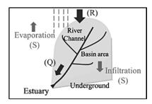
Figure 5. Concept of water balance
