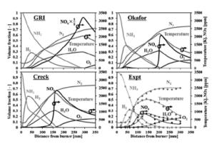
Figure 2. Flame structure at central axes of flame
