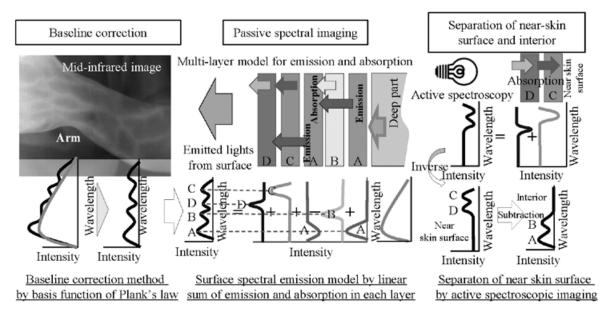
Figure 2. Conceptual diagram of analyzing spectrum of each layer from detected emission spectroscopic data radiated from skin surface.
