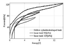
Figure 8. Energy characteristics of multi-layered variable volume tank.
