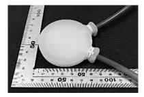
Figure 1. Hollow cylindrical-shaped variable volume tank
