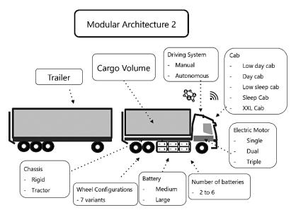
Figure 7 High level modular architecture - 2<sup>nd</sup> version
