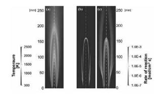
Figure 2. Calculation results. ((a) temperature, (b) rate of  $NO_x$  formation, (c) rate of  $NO_x$  reduction)
