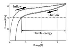
Figure 3. Energy characteristic of hollow cylindrical-shaped variable volume tank.
