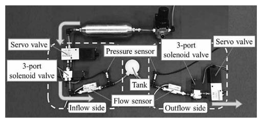
Figure 2. Experimental setup of hollow cylindrical-shaped variable volume tank.
