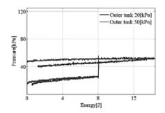
Figure 9. Relationship between pressure in the outer tank and stored energy in the inner tank.
