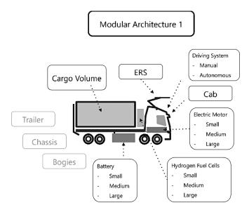
Figure 6 High level modular architecture - 1st version
