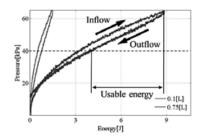
Figure 3. Energy characteristics of constant volume tank
