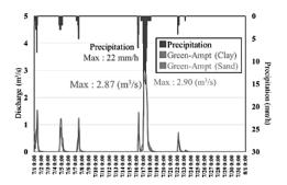
Figure 14b. Hyetograph and hydrograph (June, 2015)
