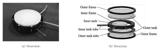
Figure 5. Multi-layered variable volume tank.
