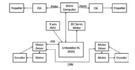
Figure 2. System configuration for Prototype 2  $\,$
