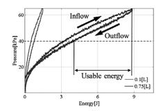
Figure 4. Energy characteristics of constant volume tank.
