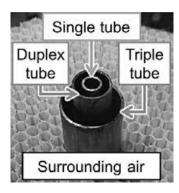
Figure 1. Burner structure (center tube:  $NH_3$ , duplex tube:  $H_2$ , triple tube: air with high velocity) .
