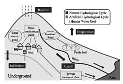
Figure 4. Interpretation of natural and artificial hydrological cycle
