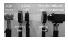
Fig 1. Optical configuration of one-shottype spectroscopy for ethanol and glucose in liquid cell.
