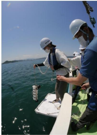
Water sampling by Van Dorm Sampler.
