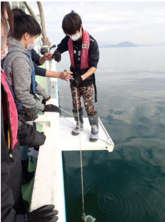
Collecting middle layer water was used the Van Dorn Water Sampler.
